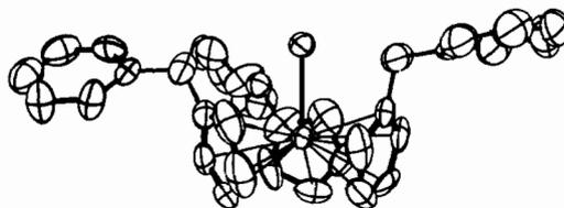
Figure 4. The  $U(C_5H_4CH_2C_6H_5)_3Cl$  molecule viewed perpendicular to the U–Cl bond (from Leong, Hodgson and Raymond,<sup>21</sup> by courtesy of the *American Chemical Society*).
