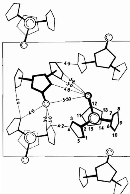
Figure 1. The structure of  $U(\pi-C_5H_5)_3Cl$  viewed down the axis (from Wong, Yen and Lee,<sup>7</sup> by courtesy of *Acta Crystallographica*).
